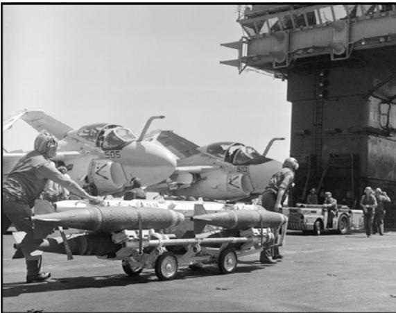
*Fig. 159: Moving Mk-82 500-pound bombs past two parked A-6 Intruder attack aircraft.*
